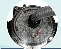
Transparent acrylic top cover provides a clear view in the filter bucket Suction hose is wrapped at the end to prevent clogging
