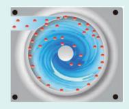
times to clean the tank, in turn minimizing the operating costs. It helps to improve machining accuracy and prevent damage to the machining surface of equipment. The cyclone effect eliminates the need to replace filter core; i.e., no consumable material needed. No bubbles are formed as it does not blend in air.
